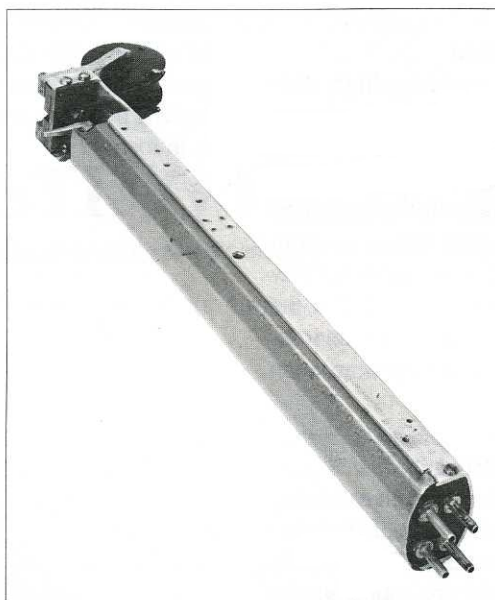
The replica of the Maxfield and Harrison wax recorder built by the author
